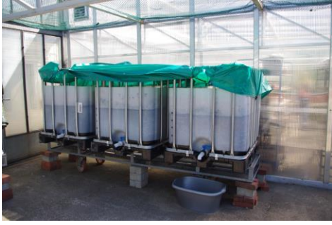
Fig. 1. Anaerobic biobed system(each container 1m 3 )
